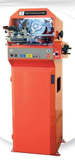
ROTAMASTER ensures both ends of a rotary blade are sharpened equally with the precision that only an automated machine can deliver. Blades have a superior edge and a consistent balance which delivers a better quality of cut, resulting in longer lasting blades and better looking grass.
