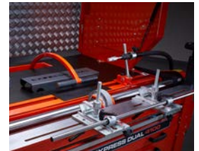
Powered clamp, reel cable drive and improved positioning scales
