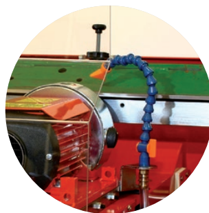
Flood coolant system comes complete with debris separation
