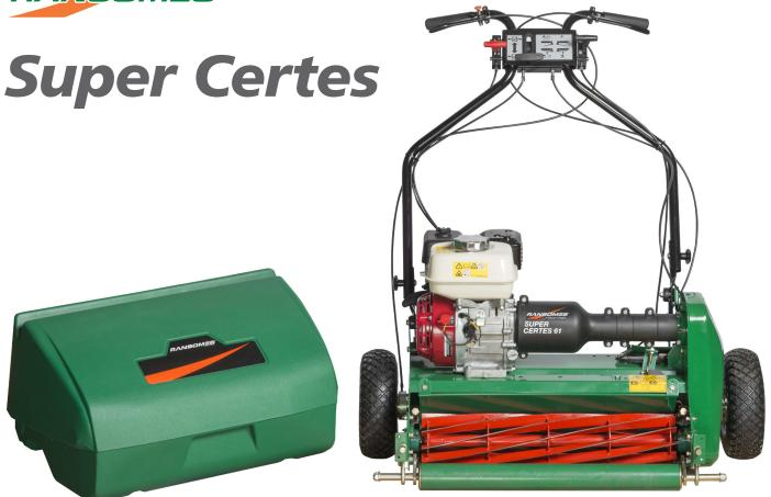
With its unrivalled reputation for precision mowing, the Super Certes is ideal for golf greens, cricket squares and grass tennis courts. Its ten blade cutting cylinder delivers 142 cuts per metre ensuring an immaculate uniform finish.
