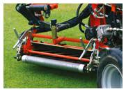
Unique swing out center cutting unit for ease of service
